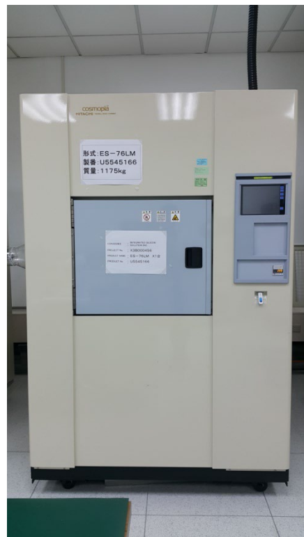
Figure 4. HITACHI Thermal Shock chamber for TCT test
