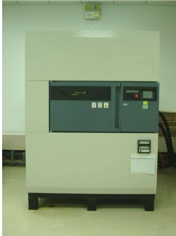
Figure 5. HITACHI Cycling Oven, for TCT test
