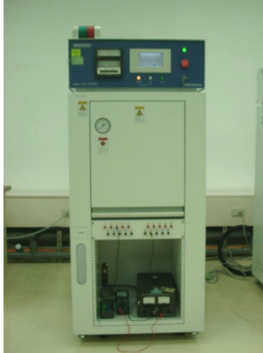
Figure 3. HIRAYAMA Pressure Oven, for HAST test
