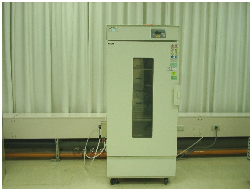
Figure 6. ISUZU High Temp Oven, for HTS test
