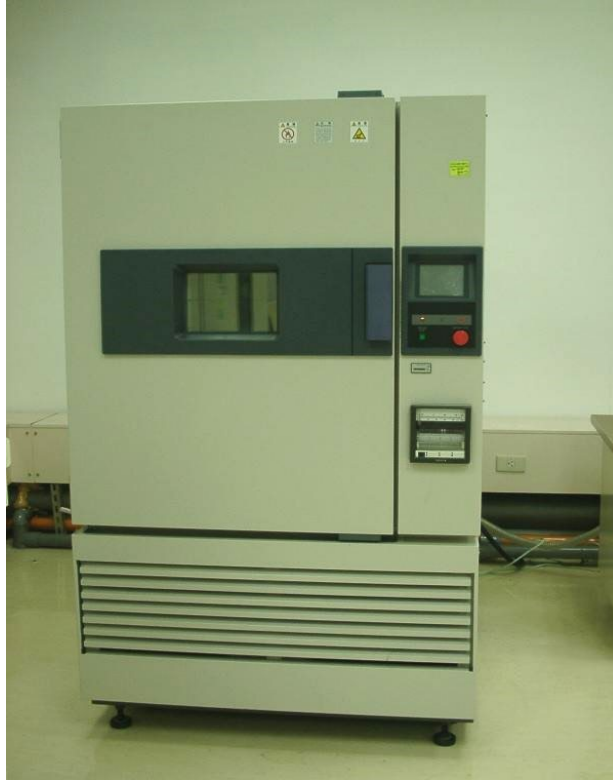
Figure 7. HITACHI Humidity Oven, for THS test
