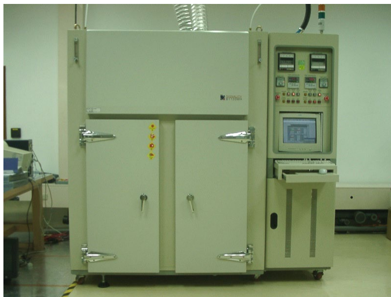
Figure 2. Signality Burn-in Oven, for HTOL test
