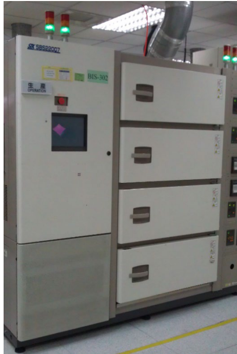
Figure 1. STK Burn-in Oven, for HTOL test
